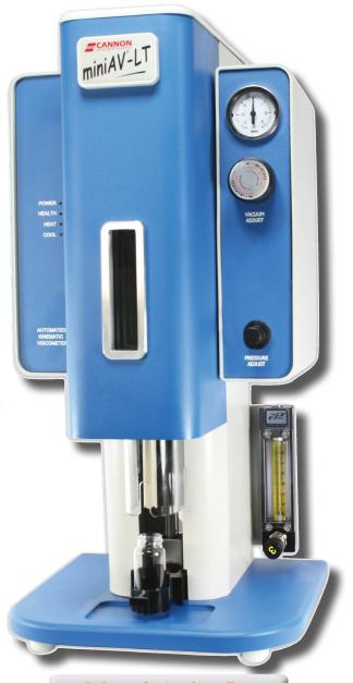
Includes professional installation, VISCPRO° data storage and management software, viscometer tube, standards, and a high precision digital thermometer
