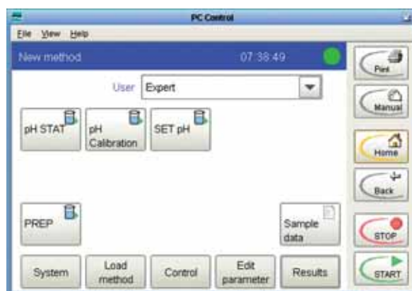
Start your titration at the push of a button: Routine methods can be linked to a «Favorite» icon on the starting screen of the 840 Touch Control.
