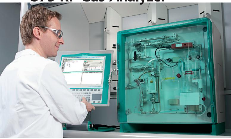
Coulometric water determination in liquid and permanent gases
