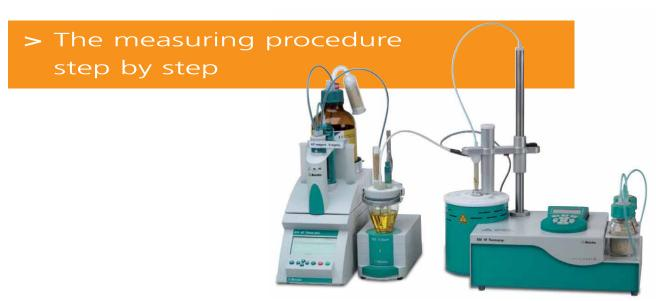
The sample is weighed into a sample vial and hermetically sealed. After the desired temperature has been reached and the titration cell conditioned, the determination is started at the KF coulometer (or KF titrator). The vessel containing the sample to be analyzed is positioned in the oven and the needle inserted through the septum of the sample vial.
